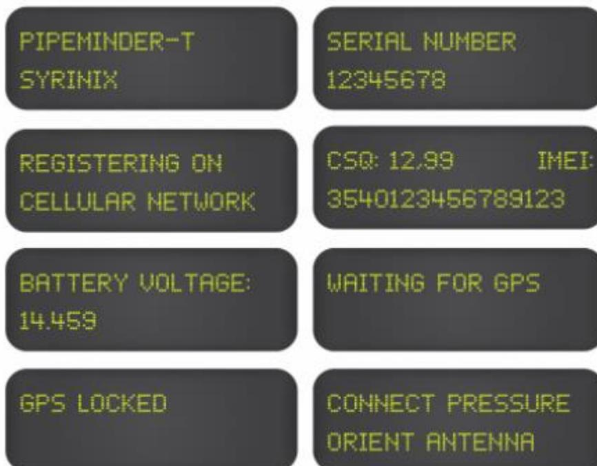
2. Once start up sequence is complete the screen will go blank please validate deployment on the RADAR cloud based platform.
