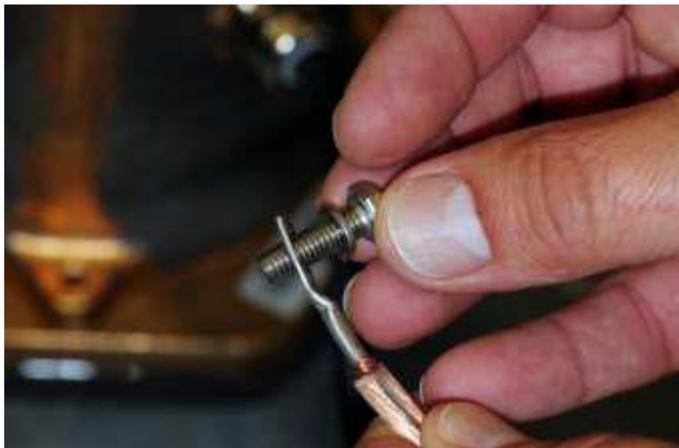
4. Replace the bolt and tighten using an appropriate socket. Do not over tighten as the screw thread in the sensor head could be damaged. Figure 10.
