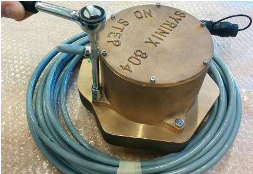
3. The earth cable should be terminated in an M6 eye tag; this is fitted to the securing bolt as shown. Figure 9.
